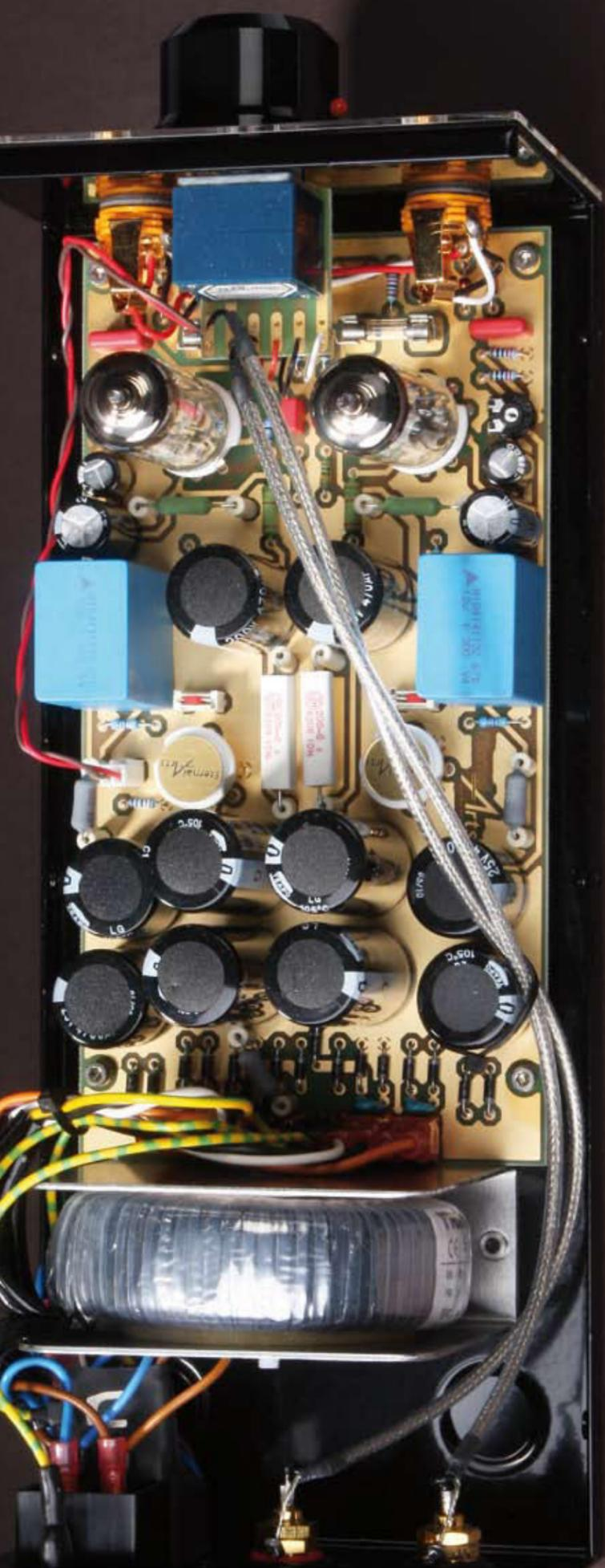
**Delicatessen – almost in full size: The main part of the sound work is carried out by two triode-pentodes immediately behind the front and ALPS pot. Very small in the middle: two (red) micro switches – to allow the use of low-ohmic headphones.**
