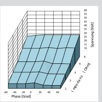
Surprisingly high output voltage if load does not fall below 6 Ohm. Very stable against phase shifts. Slight output power decrease with 2-4 Ohm loads.
